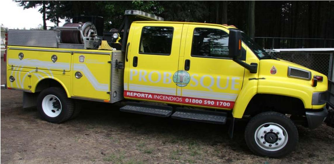
ProBosque has a single fire truck, pictured above, which we saw the very last day of our trip at ProBosque headquarters. Although the truck is approximately three years old, its use has been quite limited and its been driven very few miles. The hose on the truck was new; the truck didn't have much of a hose complement; it had only one nozzle; and it was lacking hose clamps, wyes, tees or other hardware commonly found on pumpers in the US.
