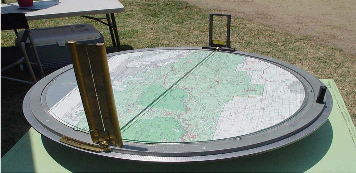
An even superior method of identifying the location of a fire is by having two or more Lookout Towers use the intersection method to fix the precise location of the fire. Using the same map at dispatch, dispatchers can then note the location of the fire and assign firefighters as needed.
